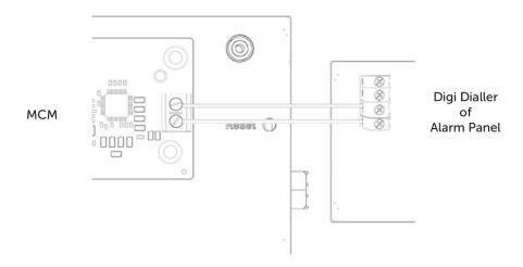
The DualCom Pro uses one of its outputs to signal the status of the Alarm Transmission System (ATS) to the alarm panel.
