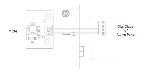
The DualCom Pro uses one of its outputs to signal the status of the Alarm Transmission System (ATS) to the alarm panel.
