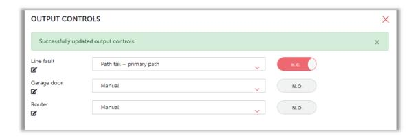
If the status cannot be obtained it will be shown on the screen. This is likely to be because the device is not currently online, or the user has pushed the N.O/N.C button several times in quick succession.
