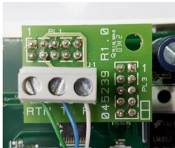
DualCom Pro ION Interface Adaptor situated on the panel
